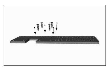
**Optional:** Use mounting plate to attach Model TAB004KL-B and other products as shown.
