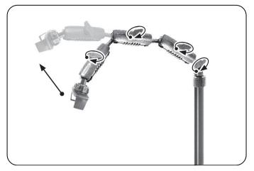
Adjust the height of the pole by loosening the adjustment collar counterclockwise. Tighten clockwise to set height.
