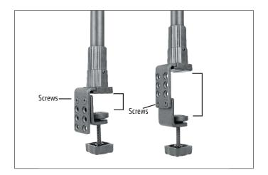
Attach overhead arm assembly to clamp pedestal by unscrewing the collar at the top of the pole until the metal ball side of the overhead arm assembly fits into the collar. Tighten collar clockwise to secure.
