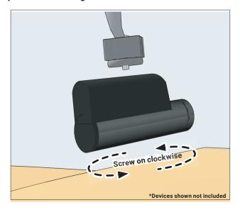
2 Attach the mount to windshield and engage Suction Lock Lever; adjust the Tightening Ring and Arm Knob as necessary
