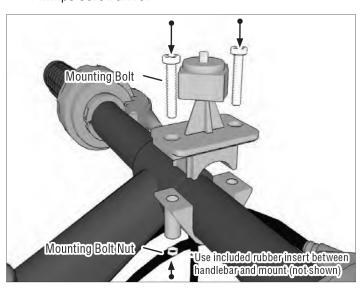
2 Attach camera or other device with 1/4" 20 mounting pattern to mounting screw on the mount
