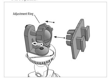
**3** Attach the Mega Grip Universal smartphone holder by sliding the Dual T-Tabs of the adapter in to the Dual T-Slots of the holder.
