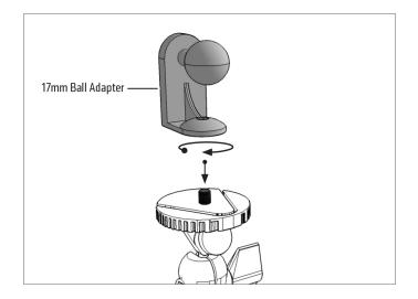
2 Attach the 17mm ball to Dual T-Tab adapter by placing the adjustment ring over the pedestal ball then snapping the adapter onto the pedestal.
