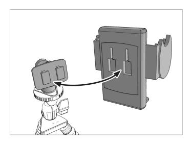
4 Adjust the removable support legs if necessary. Place device on support legs and squeeze side grip arms until they securely fit the device. Loosen adjustment ring to change the mount position.
