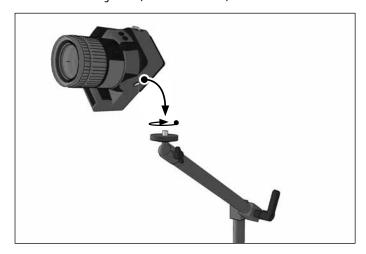
**3** Adjust the mount position by loosening the joint adjustment knobs and retightening in the desired position.
