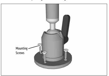
2 Attach camera or other device with ¼" 20 mounting pattern to the mounting screw (device not included).
