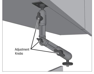
3 Attach camera or other device with <sup>1</sup>/<sub>4</sub>" 20 mounting pattern to the mounting screw (device not included).
