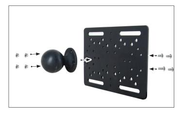
2 FLIFT57MM includes two metal mounting plates for placement on either side of the forklift guard. Use the included 3/8-16 x 4" Tap Bolts with washers and nuts to secure the plates at each corner. Use other hardware as needed for mounts or devices to the plate (devices not included).
