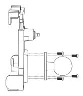
2 Installing the 38mm ball mount to the base plate
