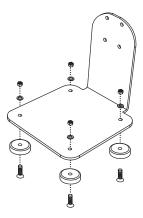
Installing the Locking Tablet holder to the shaft arm
