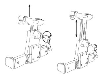
**Cocking the tablet into the holder**Firstly, place the tablet in the holder. Next, adjust the top of the holder to ensure that the tablet fits properly. Finally, press the button located at the back of the holder to lock the tablet securely in place.
