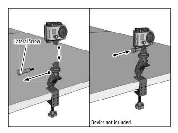
**2** Screw the GoPro adapter onto the mount's 1/4"-20 bolt.
