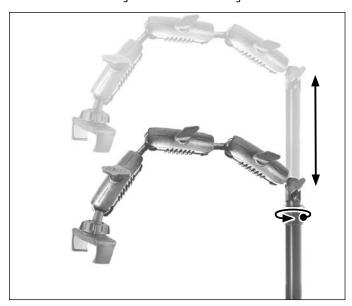
8 To maintain stability and to prevent tipping when used in the overhead view position, position the 3-shaft top arm assembly out over one of the four corners of the weighted base, not out over one of the four sides.
