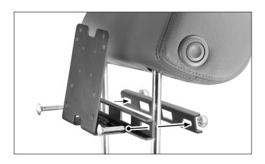
3 Attach any AMPS-compatible device (tablet, mobile printer, payment terminal; not included, sold separately) with screws and bolts.
