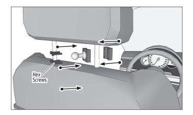
Attach 4-Hole AMPS compatible holder or device (not included).
