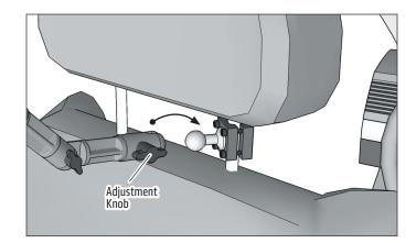
**3** Attach 4-Hole AMPS compatible holder or device (not included).
