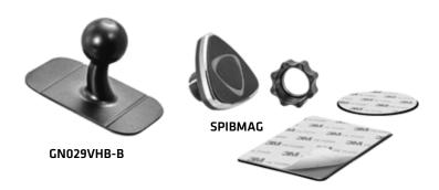
1 To attach magnet kit to adhesive adapter, slide ring over 17mm ball, snap magnetic head onto ball. Adjust angle and tighten adjustment ring to secure. Remove paper backing of adhesive metal plate. Firmly press the adhesive side to clean, back surface of your smartphone, case, or other device.
