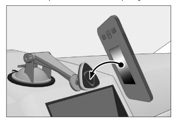
Attach pedestal to windshield or dashboard and engage suction lock lever
