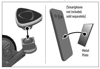
Place metal plate on the smartphone in contact with the magnet head on the pedestal to attach. Rotate or adjust angle as needed.
