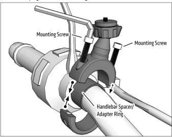
Adjust camera position as desired. Tighten adjustment ring to secure position.
