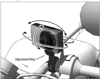
**2** Attach camera by screwing it onto the 1/4"-20 mounting bolt.
