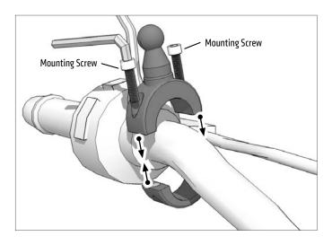
**3** Unscrew lateral screw and insert GoPro into GoPro mounting pattern. Reinsert lateral screw and tighten to set.
