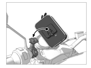
Insert device and adjust holder (sold separately, not included) position as desired. Tighten adjustment ring to secure position.
