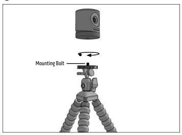
**2** Loosen the adjustment knob to change position. Retighten to set.
