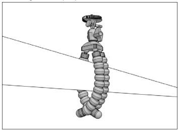
Release the 1/4"-20 mount by unscrewing lateral screw and pressing on release tab.
