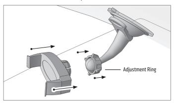
**OPTIONAL:** For semi-permanent dashboard installation, use included adhesive mounting disk\*.
