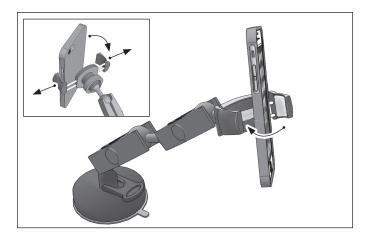
To add phone holder, place tightening ring over 17mm end of ball adapter and snap the Mobile Grip Holder onto adapter. Set to desired position and tighten ring.
