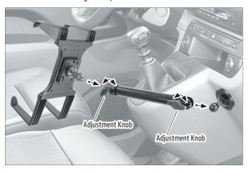
**2 C**) Attach the square AMPS adapter to the holder with the provided screws. **D**) Select a safe location in the vehicle to drill and install the round drill base adapter with the provided screws or with your own screws.
