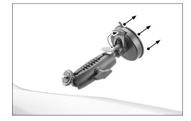
**3** Attach camera (not included, sold separately) by screwing the camera onto the 1/4"-20 mounting bolt.
