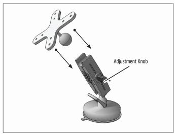
3 Attach any VESA 75/VESA 100 compatible device or holder (not included, sold separately) to the VESA plate. Loosen adjustment knob to adjust angle of pedestal and position of VESA plate. Tighten to secure.
