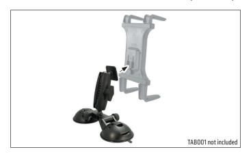
2 Clean mounting area thoroughly with included alcohol pad and let dry. Remove the protective film from each of the suction cups. With the tabs on the suction mounts UP, place mount on windshield then flip tabs DOWN to engage suction.
