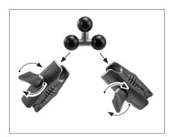
Attach Robust mount shaft **SP-RMS250 to SPRM080** by loosening adjustment knob to adjust position. Retighten to set.
