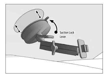
2 Attach Slim-Grip Ultra holder by sliding the Dual T-Tabs on the pedestal head into the Dual T-Slots of the holder.
