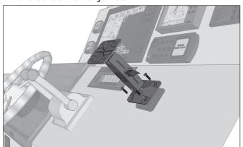
Attach your electronic fishfinder or other marine radio to the mounting plate through the AMPS base plate. Choose the screws (not included) that will work best to mount your device.
