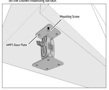
2 Attach any AMPS-compatible device, holder, or adapter (not included, sold separately) to the AMPS adapter plate.
