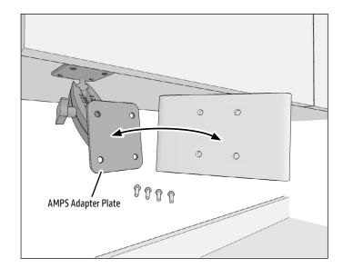
3 Loosen adjustment knob to adjust position. Retighten to set.
