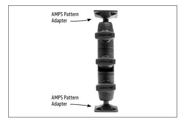
To adjust the angle of the center robust ratcheting elbow, loosen the center adjustment knob. Retighten the knob desired angle. The angles of the 4-hole AMPS pattern mount can also adjusted using the adjustment knobs directly above the 4-hole AMPS pattern adapter plates.
