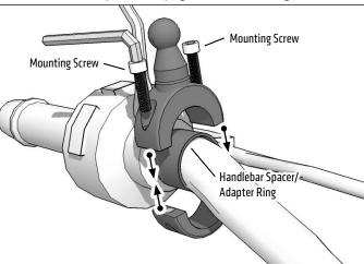
2 Place adjustment ring over the mount's ball. Snap the RoadVise Holder onto the mount and tighten adjustment ring to set position.
