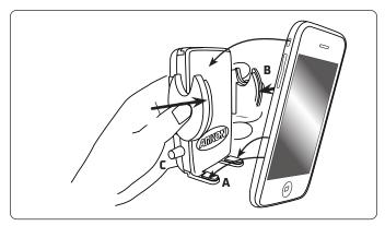
3 Push the release button (C) to open the side grip arms and remove the device.
