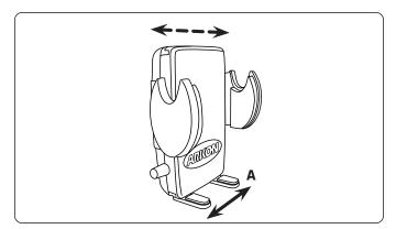
2 Place device on the support legs (A) and squeeze the side grip arms (B) until they fit securely to the device.
