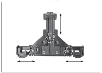
2 Insert device and push down on the center arm.
