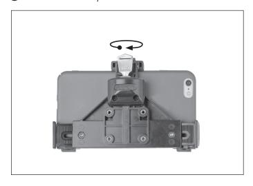
4 Attach AMPS compatible adapter to back with included screws.
