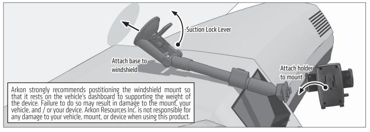
2 Adjust length of mount as necessary by unlocking extension arm. Lock arm when desired length reached. Insert device by pushing release button to release the arms. Adjust legs to desired position. Insert device and close arms to secure.
