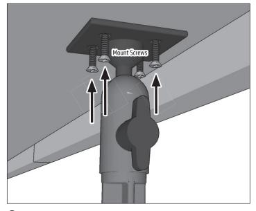
3 Attach device holder to mount by inserting screws through adapter into the screw openings in the device holder.
