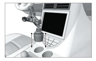
(A) Use a Phillips screwdriver to loosen the 3 screws to adjust the holder to the size of your device. Tighten screws to set. (B) Insert device and push down on the center arm. (C) Lock with included key.
