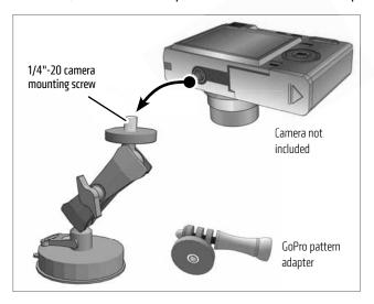
Remove screw from the 3-prong bracket and insert GoPro camera and case, then re-insert screw. Tighten and rotate as needed.
