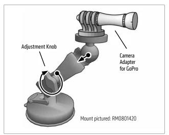
**OPTIONAL:** To attach any small action camera with a 1/4"-20 mount connection, unscrew the GoPro pattern end of the 25mm ball adapter.
