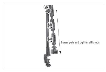
4 Adjust the height of the pole by loosening the adjustment collar. Tighten at desired height.
