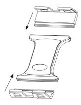
Install the tablet With the holder's spring-loaded support legs expanded, lay the tablet flat on the holder.
