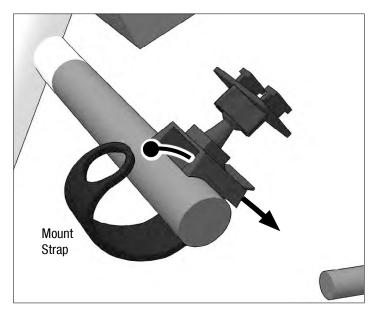
**3** Place device in the holder by pushing down on holder's lower legs.
