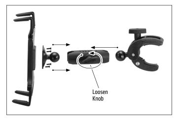
**3** Tighten clamp knob to mount to pole or surface.
