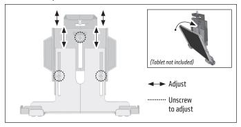
**6** To lock down tablet, close down on the locking arm on the top of the tablet and lock with key (included).
