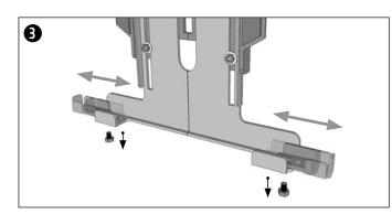
Unscrew the screws at the bottom sides of the holder to adjust the tablet holder's width to the tablet. Tighten to secure.
