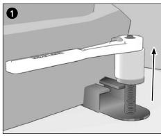
Use a socket wrench to loosen the passenger seat track bolt.
