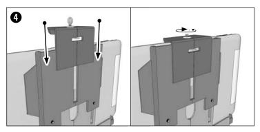
To lock down tablet, close down on the locking arm on the top of the tablet and lock with key (included).
