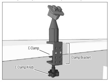
Insert the tablet holder's Dual T-Slots into the mount's Dual T-Tab head.
