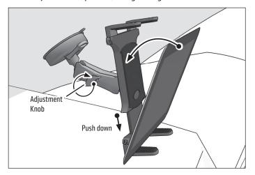
2 Attach Slim-Grip tablet holder by sliding the Dual T-Tabs of the pedestal head into the Dual T-Slots of the holder.
