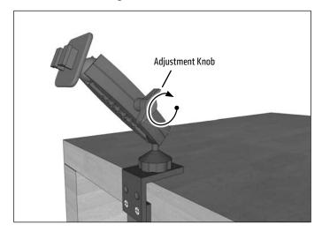
4 Insert tablet by placing it on the two lower legs and pushing down on the spring-loaded bottom of the holder. Loosen adjustment knob to adjust rotation, position, or angle. Retighten to set.
