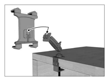
Loosen adjustment knob to adjust position. Retighten to set to desired angle.
