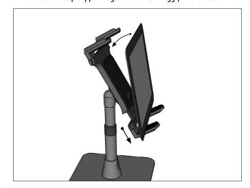
Adjust the height and angle of the pedestal by loosening the adjustment ring and the adjustment knob. Retighten to set.
