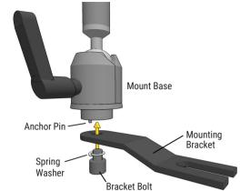
Loosen the passenger seat track bolt with a socket wrench and insert the mounting bracket between the bolt and the seat track; firmly retighten the seat track bolt.
