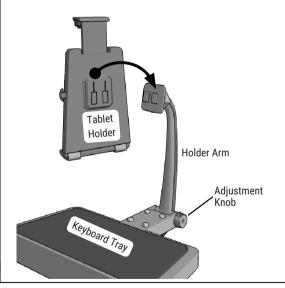
Insert tablet into holder and place keyboard on the tray.
